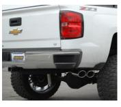
8. Install stainless steel tip. Clamp down. When you have everything in place, firmly tighten all bolts and clamps down securely. Use stainless steel cleaner weekly to prevent tip from discoloration. Inspect all fasteners after 25-50 miles of operation and re-tighten as necessary.
